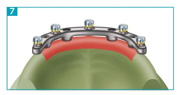
7 Snap a Denture Housing with a Yellow Processing Male onto each LOCATOR Bar Abutment and verify that the laser weld does not interfere with the Housing seating completely.
