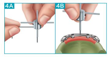
**4A-4B** Divest, finish and polish the cast bar. Finger tighten the Bar Tap manually into the Drill and Tap Holder. Use the Bar Tap to manually chase and clean the internal threads of each insert.
