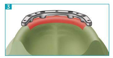
3 Invest and cast the bar using standard casting procedures. The threaded inserts will become part of the cast bar.
