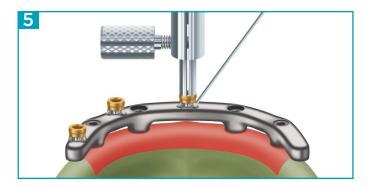
5 Place the Paralleling Mandrel in a surveyor and place the LOCATOR Bar Abutments in position on the bar. Tack the LOCATOR Bar Abutments into place by spot welding on opposite sides.
