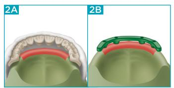
**2A-2B** With the teeth placed back in the matrix, seat the matrix on the model. Determine the locations for the LOCATOR Bar Abutments in relation to the implant positions, spacing between attachments and the interarch space. Wax the overdenture bar to the implant components.
